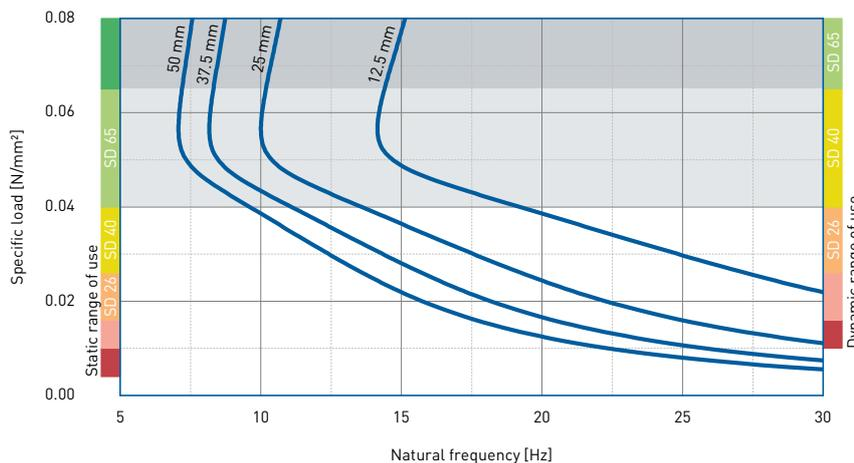
Natural frequency of a single-degree-of-freedom system consisting of a fixed mass and an elastic bearing consisting of PURASYS **vibrafoam** SD 40 on a stiff subgrade.
